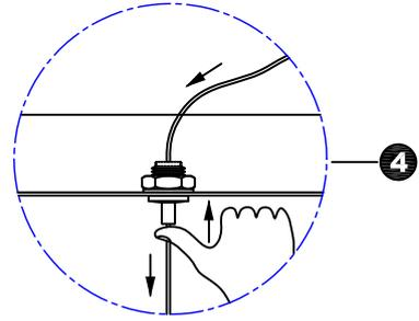
**Note:** Press the wire restraint to adjust the desired length of cable.
